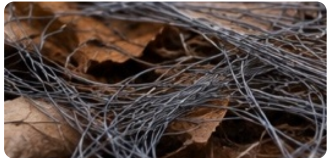
Close-up of the weave: wire of 0.5–0.9 mm diameter in four rows of rings.
